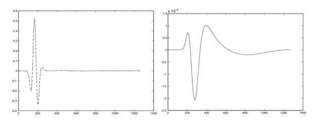
Figure 3: Pressure field (left) and error on the pressure (right) near the upper left corner for an oblique velocity M=0.9 vs. time steps
